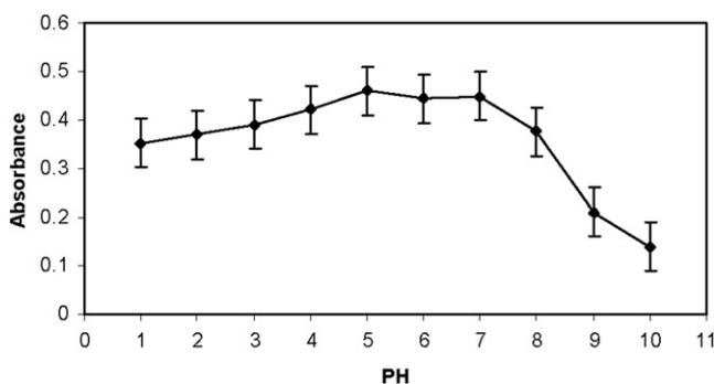
Figure 5. Effect of pH on the absorbance of arsenic obtained from DLLME. Extraction conditions, as with Figure 3; extraction solvent (1-undecanol) volume, 45  $\mu\text{L}$ .
