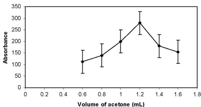
Figure 4. Effect of the volume of the disperser solvent (acetone) on the absorbance of arsenic obtained from DLLME. Extraction conditions, as with Figure 3; extraction solvent (1-undecanol) volume, 45  $\mu$ L.
