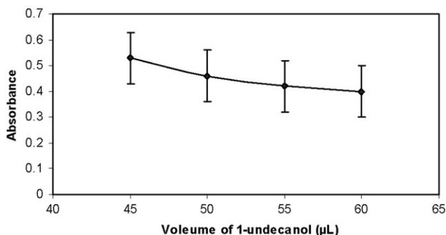
Figure 3. Effect of the volume of extraction solvent (1-undecanol) on the absorbance of arsenic obtained from DLLME. Extraction conditions: water sample volume, 9.8 mL; disperser solvent (acetone) volume, 1.20 mL; APDC amount, 10 mg; pH 6.00; As(III) concentration, 5 µg L<sup>-1</sup>.
