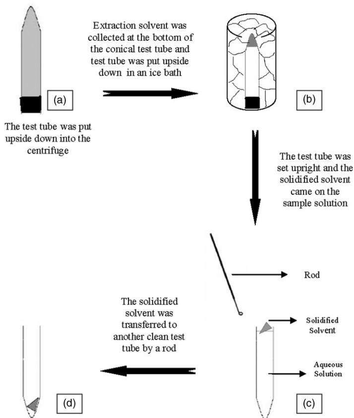
Figure 1. Schematic diagram of the proposed DLLME procedure.
