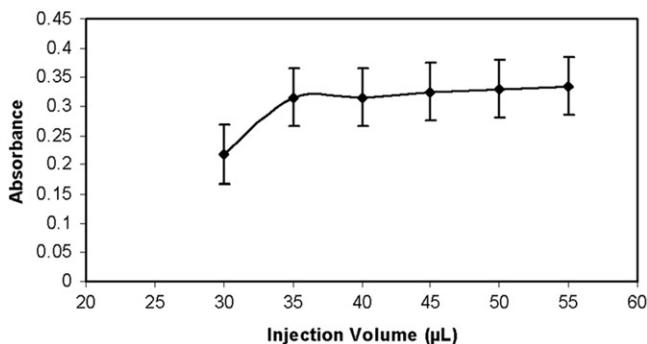
Figure 2. Effect of the injection volume on the signal height. (Extraction conditions have been mentioned in section 2.4.)
